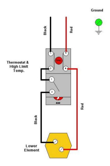
S Model Double Element Configuration with Mechanical Thermostats Simultaneous Operation (#6 Wiring)
