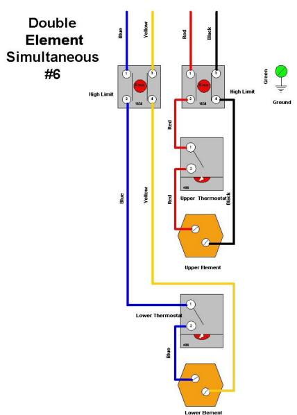
S Model Double Element Configuration with Mechanical Thermostats Simultaneous Operation (High Temperature Usage)
